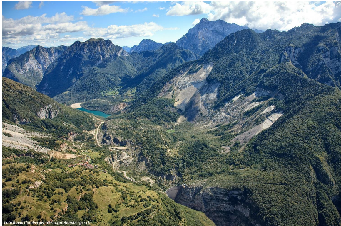
Figure 1: Aerial oblique view (upstream) of the Vajont slide; in the foreground the dam, Monte Toc and sliding plane to the right, rest of the reservoir in the background; From [12].
